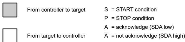
**Figure 9-8. Legend for the I<sup>2</sup>C Sequence Diagrams**
