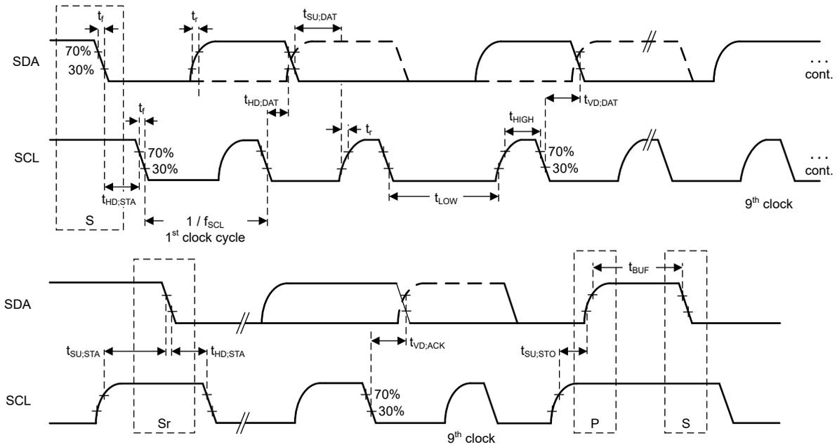
**Figure 6-1. I<sup>2</sup>C Timing Requirements**
