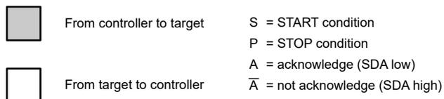
**Figure 7-11. Legend for the I<sup>2</sup>C Sequence Diagrams**
