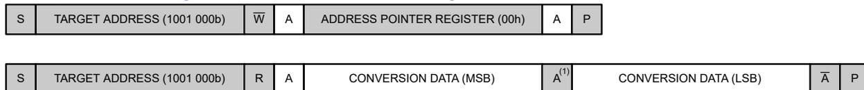
**Figure 9-7. Read the Conversion Register**
